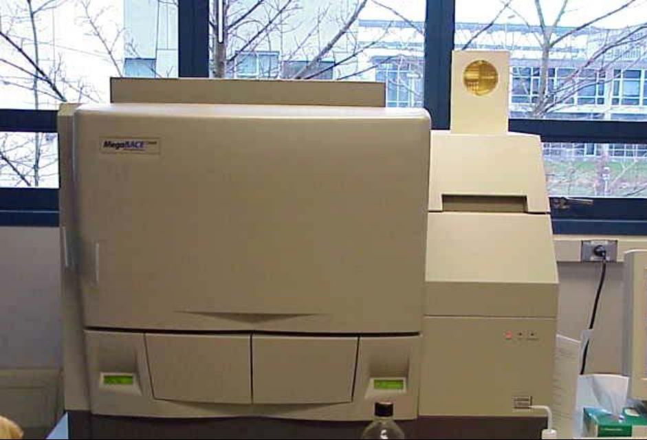
Megabase Sequencer that analyzes 96 sequencing reactions at a time
