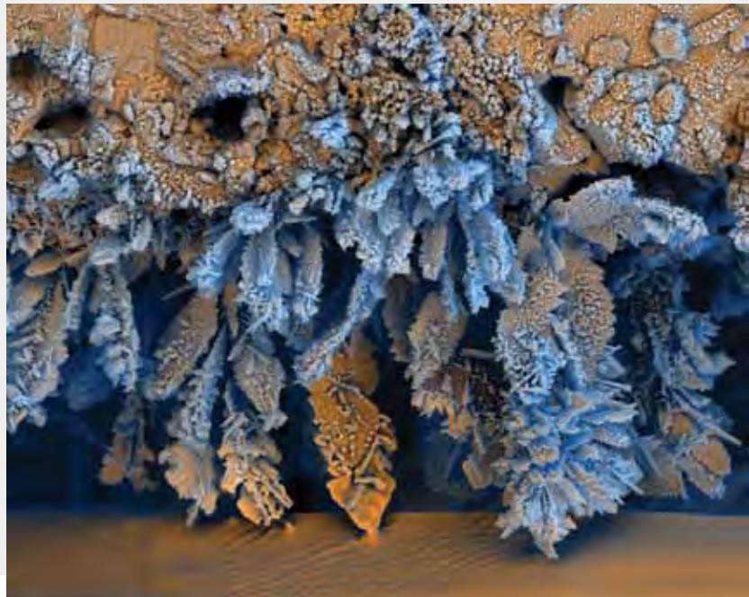
Automotive light bulb analysis to determine failure, imaged on an SEM.
