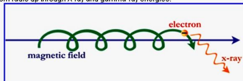
Synchrotron Radiation: Electrons moving in magnetic field radiate photons.
