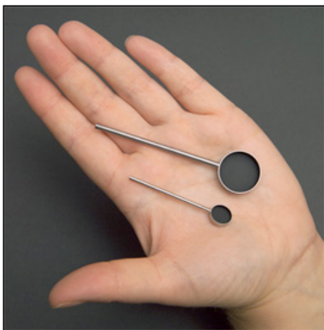
The iTC 200 utilizes a 200 \mu l cell versus the 1.4 ml cell in previous models.
