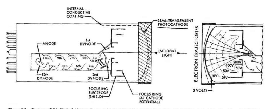
Figure 3-8. Beckman-RCA Bialkali 12-stage Photomultiplier Tube. (Courtesy of Beckman Instruments, Inc., Instruction Manual 1553-D.)
