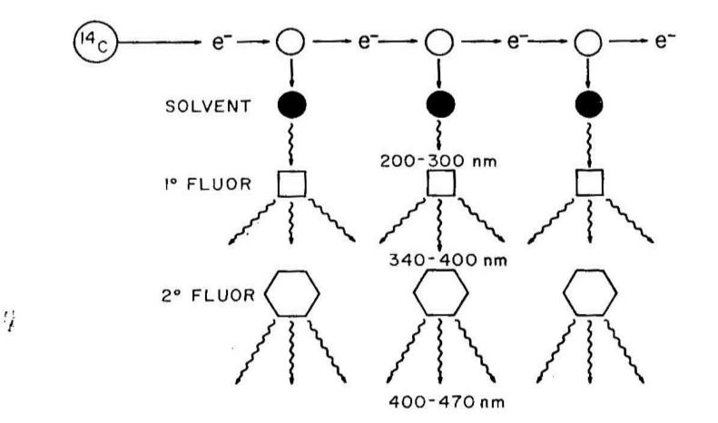
Figure 3-2. Interaction of  $\beta$  particles with aromatic solvents and subsequent fluor excitation.  $e^-$  represents the emitted  $\beta$  particles,  $\bigcirc$  indicates a solvent molecule in its ground state, and  $\bigcirc$  denotes solvent molecules in the triplet state. (From E. Rapkin, *Preparation of Samples for Liquid Scintillation Counting*, Picker Nuclear Corp., White Plains, New York.)
