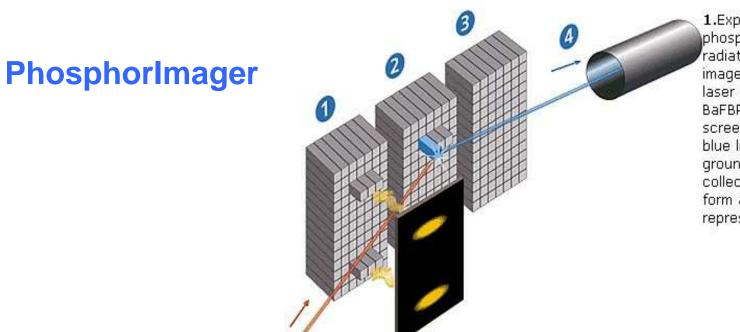
1.Exposure of the storage phosphor screen to ionizing radiation induces latent image formation 2. During laser scanning, the BaFBR:EU+2 crystals in the screen release energy as blue light 3. and return to ground state 4. Blue light is collected and measured to form a quantitative representation of the sample.
