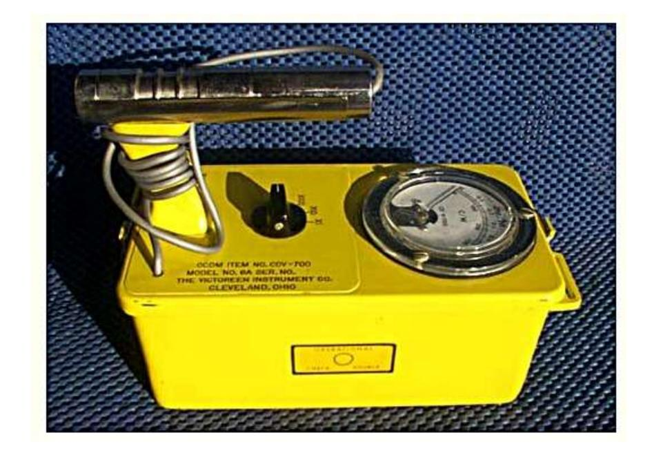
A Geiger counter depends on the fact that radiation knocks electrons out of the atoms in a gas and leaves them with an electric charge. These charged atoms (or ions) can then carry an electric current through the gas.
