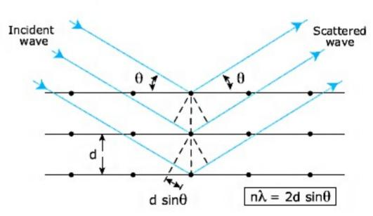
X-ray scattering from three crystal planes, separated by the distance d. For constructive interference in a direction  $\theta$  the path difference must be an even number of wavelengths.
