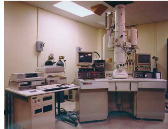
JEOL JEM-2010: 200kV high-resolution TEM with interchangeable polepieces, where one can change from an analytical version (resolution = 0.23nm, +/- 30 degrees tilt) to a high-resolution version (0.19nm, +/- 10 degrees tilt). Double-tilt and heating specimen holders are available on this TEM. http://www.tamu.edu/mic/instruments.html#jem2010
