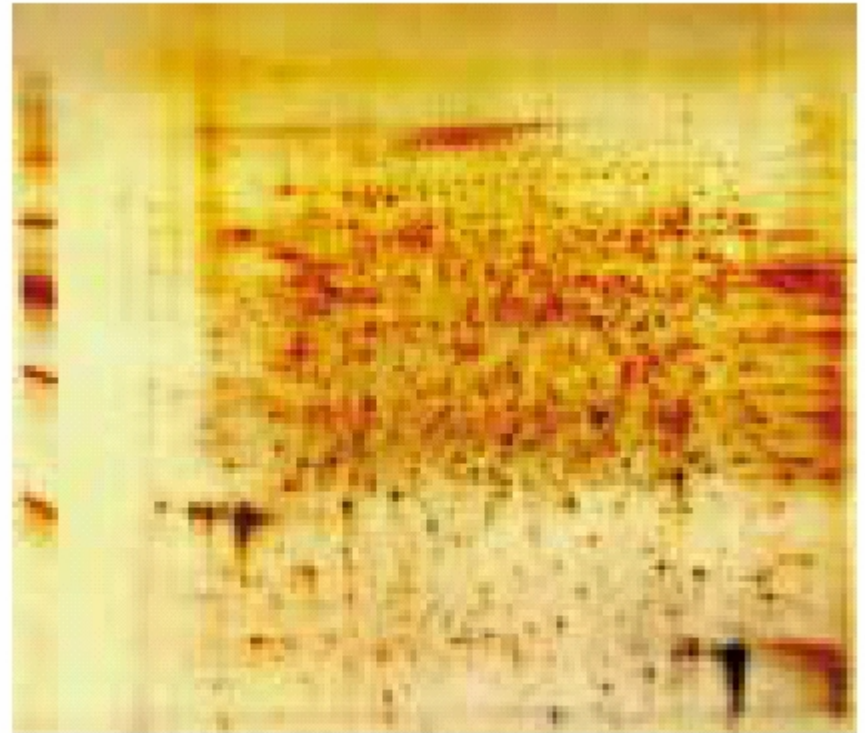
2-D electrophoresis of mouse liver proteins using 180 mm IPG strips and horizontal large scale SDS-PAGE gel, silver stained. Görg A. Biochem. Soc. Trans. 21 (1993) 130-132 With kind permission of the author.
