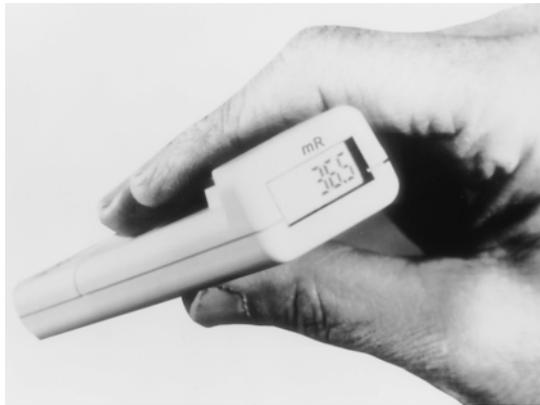
**Figure 32.** Photograph shows a pocket solid-state personnel dosimeter. This unit displays cumulative exposure in milliroentgens. (Courtesy of Nuclear Associates, Carle Place, NY.)
