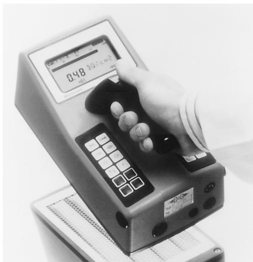
**Figure 25.** Photograph shows an extremity and area ionization detector. This unit has a large surface area and can be handheld or wall mounted for convenient monitoring of hand contamination. (Courtesy of Nuclear Associates, Carle Place, NY.)
