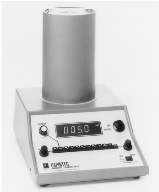
**Figure 26.** Photograph shows a nuclear medicine dose calibrator used for the assay and verification of radionuclide doses before administration to patients. The syringe containing the dose to be assayed is lowered into the center of the well-shaped containment vessel, which is filled with a high-density gas (eg, argon). The activity in millicuries or megabecquerels is read directly from the light-emitting diode readout. (Courtesy of Capintec, Ramsey, NJ.)
