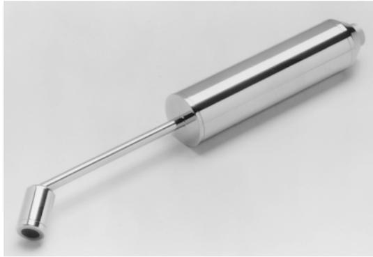
**Figure 33.** Photograph shows an intraoperative probe used for lymphoscintigraphy applications. The narrow tip contains a cadmium telluride wafer transducer and can be used with or without a collimator aperture sleeve, the need for which depends on the position discrimination and sensitivity required. (Courtesy of Radiation Monitoring Devices, Watertown, Mass.)
